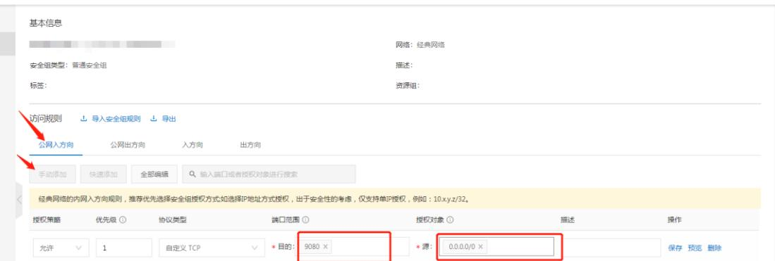
The screenshot shows a network security group configuration page. The '访问规则' (Access Rules) tab is selected. Under the '公网入方向' (Public Network Incoming Direction) section, there is a table with one row. The row details are: 操作 (Action) set to 允许 (Allow), 优先级 (Priority) set to 1, 协议类型 (Protocol Type) set to 自定义 TCP (Custom TCP), 目的 (Destination) set to 9080, and 源 (Source) set to 0.0.0.0/0. A red box highlights the destination and source fields.
