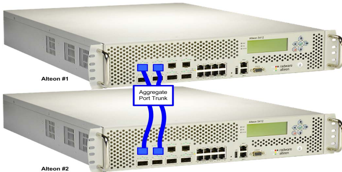
Figure 6: Example Port Trunk Group Between Alteons
